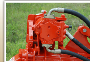
HYDROSTATIC DRIVE With 2.48ci hydrostatic motor, 8cc gear pump and 4.6ci hydrostatic transmission
