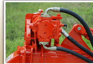
HYDROSTATIC DRIVE 2.48ci hydrostatic motor with 8cc functions gear pump, 16cc track drive gear pump and 4.6ci hydrostatic transmission
